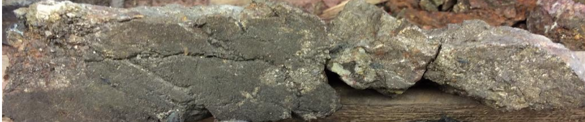
Massive sulfide mineralization (BH73004)
