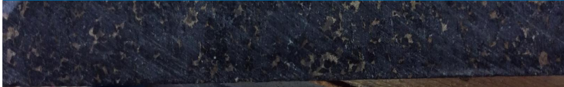
Disseminated Ni and Cu-rich sulfides in ultra-mafic intrusion (BH79018)
