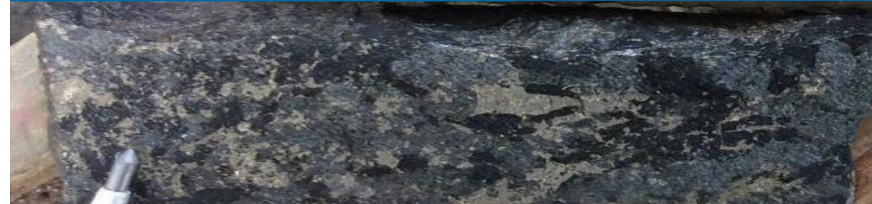
Sulfide impregnation (BH73004)
